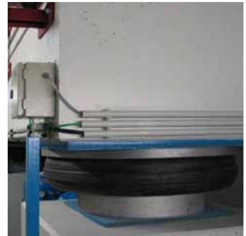
Air Spring with additional volume
